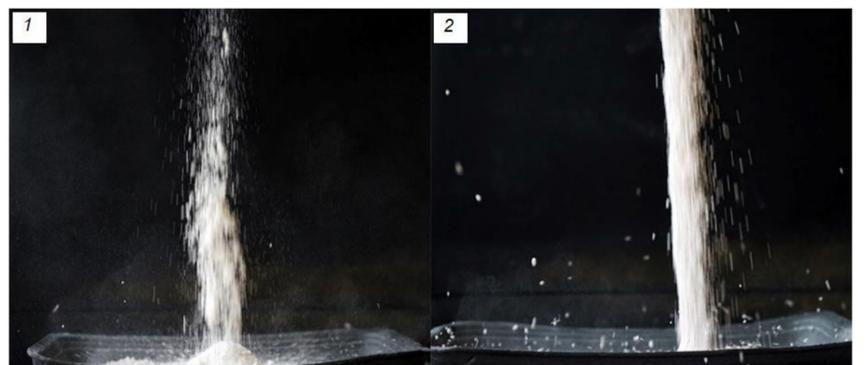
**Fig. 5.** Ca/Mg/PO<sub>4</sub> dust test: 1 – not granulated, 2 – granulated using FBG
