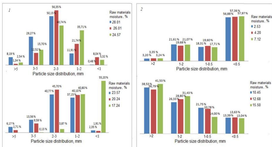
**Fig. 2.** Dependence of Ca/Mg/PO<sub>4</sub> with K and ME additives particle size distribution on raw material moisture: 1 – DG; 2 – FBG
