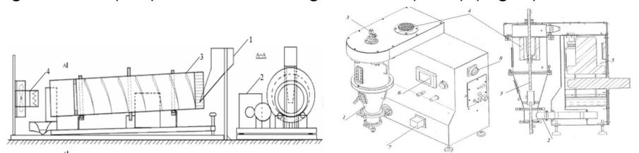
**Fig. 1.** Drum granulator and a fluid bed granulator
