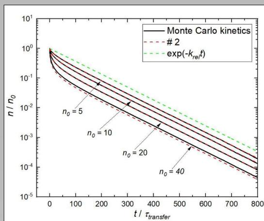
Fig. 4. Statistical approach approximation using  $\gamma(t)$  that provides the best fit.
