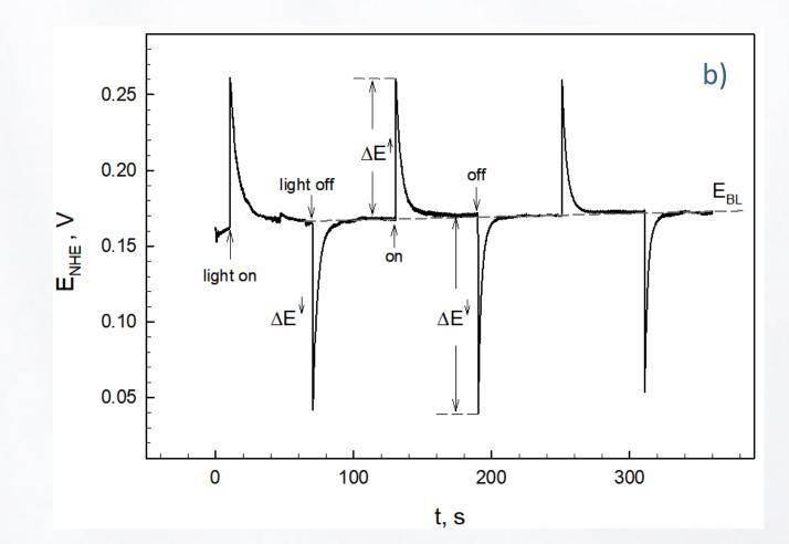
Photopotential variation at open circuit of p-Si coated with  $HfO_2$  in 1 M  $NaClO_4$  (pH 3) when illumination is chopped at 1 min intervals for 10 nm (a) and 60 nm (b)  $HfO_2$  layers on p-Si. Irradiation:  $\lambda = 505$  nm and N = 50 mW cm<sup>-2</sup>
