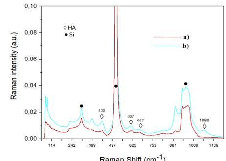
Fig. 7. Raman spectroscopy analysis shows characteristic HA peaks at 430, 607, 667, 1080  $\text{cm}^{-1}$  formed after Si substrates were stored in disodium hydrogen phosphate,  $\text{Na}_2\text{HPO}_4$  solution (1 mol/l) for 28 days in a thermostat at 80 °C, using both spin-coating techniques a) and b).
