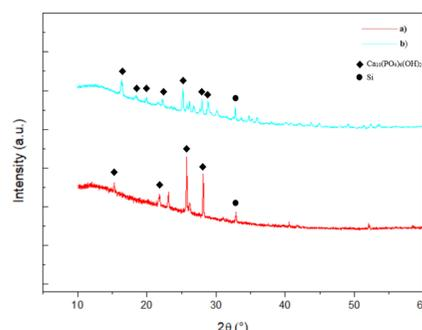
Fig. 6. XRD analysis shows characteristic HA peaks after Si substrates were stored in disodium hydrogen phosphate,  $\text{Na}_2\text{HPO}_4$  solution (1 mol/l) for 28 days in a thermostat at 80 °C, using both spin-coating techniques.
