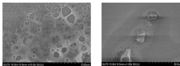
Fig. 2. SEM analysis shows single  $\text{CaCO}_3$  crystallites are formed on silicon substrate using spin-coating technique.
