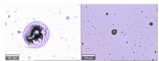
Fig. 3. Photographed on a Raman spectrometer. By pointing the laser at the individual crystallites formed, HA signals can be observed.
