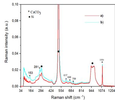
Fig. 5. Raman spectroscopy analysis shows characteristic  $\text{CaCO}_3$  peaks at 153, 281, 617, 668, 709, 1084  $\text{cm}^{-1}$  formed after 20 coatings using both spin-coating techniques a) and b).
