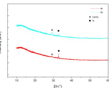
Fig. 4. XRD shows characteristic  $\text{CaCO}_3$  peaks formed after 20 coatings using both spin-coating techniques a) and b).
