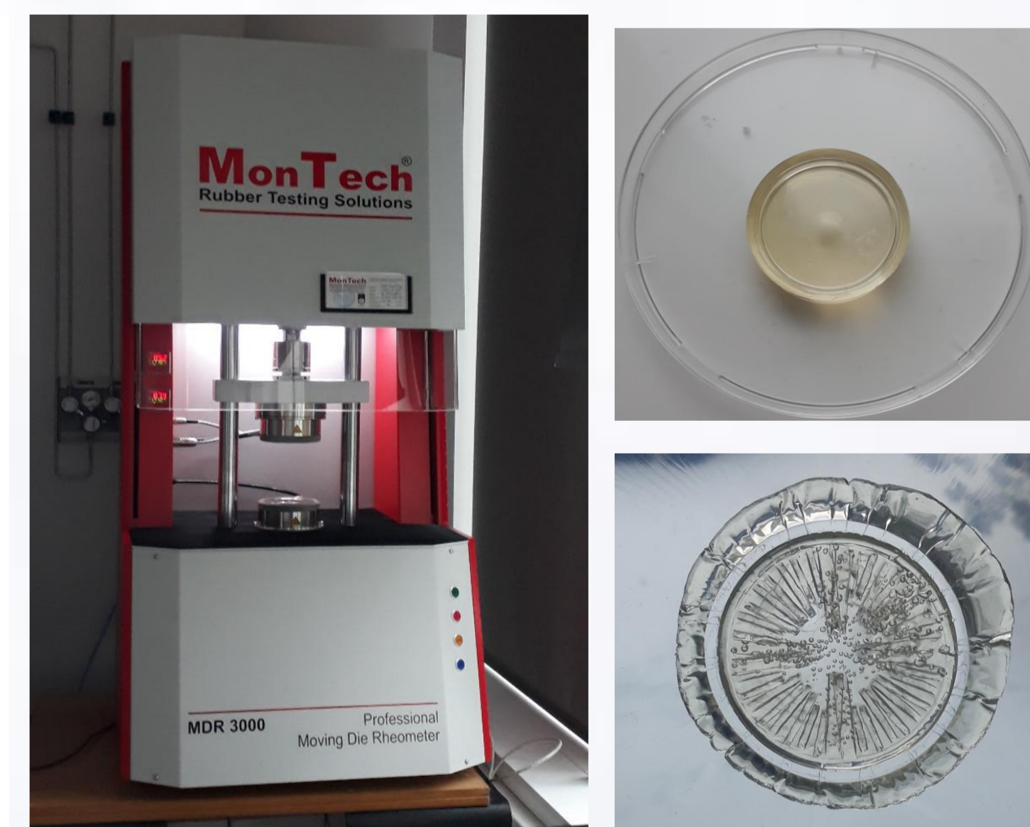
Fig. 2 D-MDR 3000 (Montech) and applied sample before and after test
